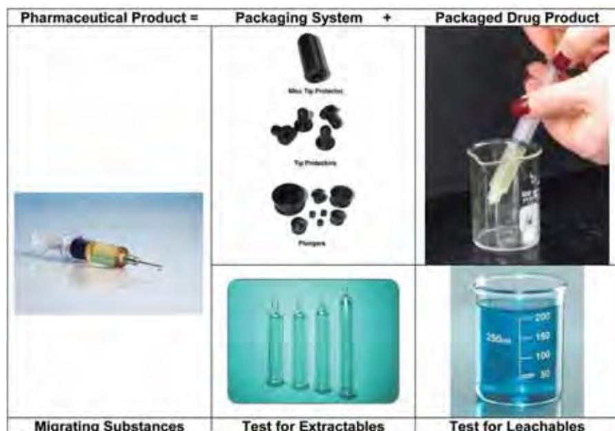
**Figure 2** Use of a pre-filled syringe to illustrate the relationship between extractables and leachables. The actual pharmaceutical product is characterised for migrating substances by either testing its packaging system for extractables or its packaged drug product for leachables
