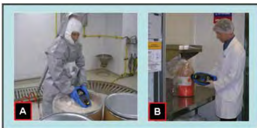
FIGURE 2 Section A: Pfizer colleague using handheld Raman instrumentation for through liner scanning in a containment facility in Puerto Rico. Section B: Pfizer colleague using similar instrumentation for through liner and container scanning in Australia
