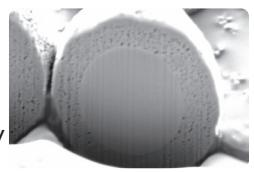
Fused-Core® particles consist of a solid silica core and a porous silica shell allowing a shorter diffusion path compared to conventional fully Porous Particles.
