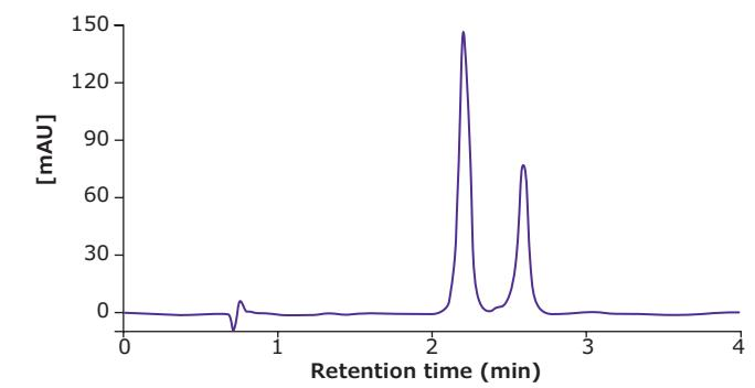
The same separation on a Chromolith® 2 mm I.D. column demonstrates improved sensitivity and solvent savings of 81 %.
