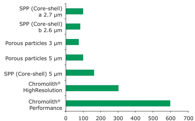
All columns are C<sub>18</sub> modified, 100-4.6 mm. Sample: anthracene, eluted isocratically using acetonitrile/water (60/40) at 2 mL/min flow rate. Injection volume: 5 µL, detection at 254 nm UV. All analyses performed at room temperature.
