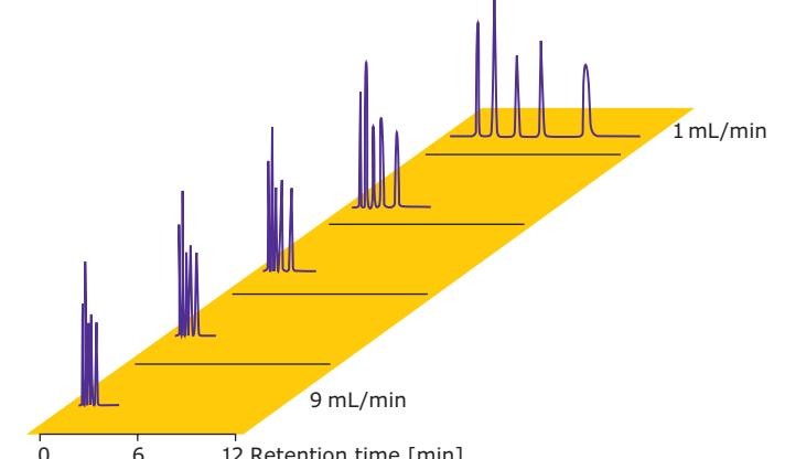
Owing to the very high porosity of the Chromolith® WP 300 column, very high flow rates can be applied with very low pressures as seen above.
