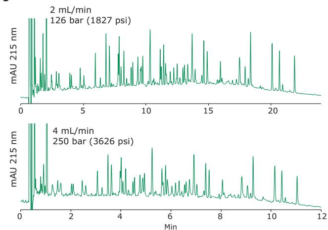
BIOshell™ A160 Peptide columns can more than double sample throughput by allowing the analyst to operate at higher flow rates without a concomitant drop in efficiency.
