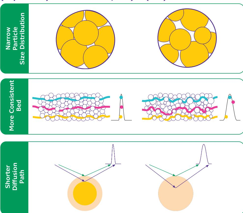
The innovative manufacturing process for Fused-Core® particles produces a very narrow particle size distribution. This allows for the use of larger porosity frits that clog less, resulting in a more rugged column. Traditional fully porous particles provide a larger particle size distribution, requiring smaller pore frits that clog more easily.
