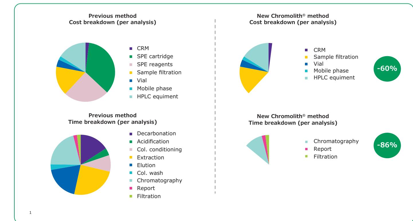
Time and cost per analysis for the determination of Iso-alpha-acids in Beer using a particulate and a monolithic column.
