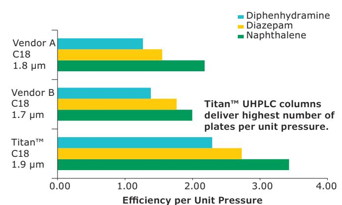
Titan™ UHPLC columns deliver highest number of plates per unit pressure.
