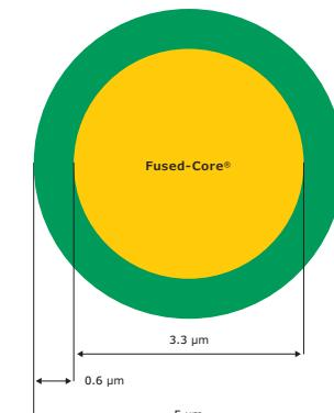
True plug and play solution for improving separations on existing 3 µm or 5 µm fully porous particle HPLC columns
