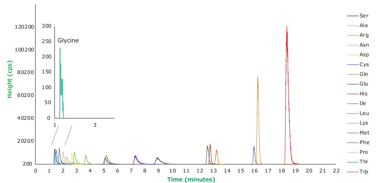
Separation of 20 underivatized amino acids by LC-MS/MS. Conditions: Column: Supel™ Carbon LC, 10 cm x 2.1 mm I.D., 2.7 µm; Mobile Phase: [A] Water (0.1% (v/v) DFA); [B] Acetonitrile (0.1% (v/v) DFA); Gradient: Hold at 0% B for 7 min; 0% B to 5% B in 5 min; 5% B to 100% B in 10 min; Flow Rate: 0.2 mL/min; Column temp.: 12 °C; Detector: MSD; Injection: 1.0 µL; Sample: Amino Acid Mix, varied concentration, water (0.1% (v/v) DFA)
