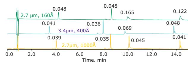
Higher efficiencies and better sensitivity can be realized with proper pore diameter selection. Here, the 1000 Å pore diameter is the only one capable of providing good peak shape of the mAb (peak 3) analyte.
