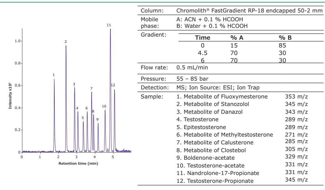
Excellent, ultra-fast results are obtained, not only in UHPLC and UPLC® instruments, but equally well in all standard HPLC systems with low dead volume. Chromolith® 2 mm columns have macropores of 1.5 µm in diameter, resulting in a column efficiency that exceeds 100,000 plates/meter.
