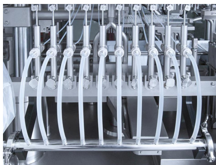
Ten rotary piston pumps. Behind the array of pumps can be seen ready-to-use containers in nest and tub format. Image courtesy of Bausch+Ströbel. Used with permission.
