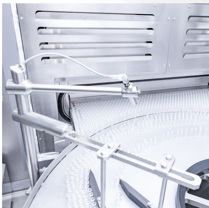
Washed and sterilized bulk vials coming out of a depyrogenation tunnel and accumulating on a rotary table prior to filling. Image courtesy of Optima Packaging Group GmbH. Used with permission.
