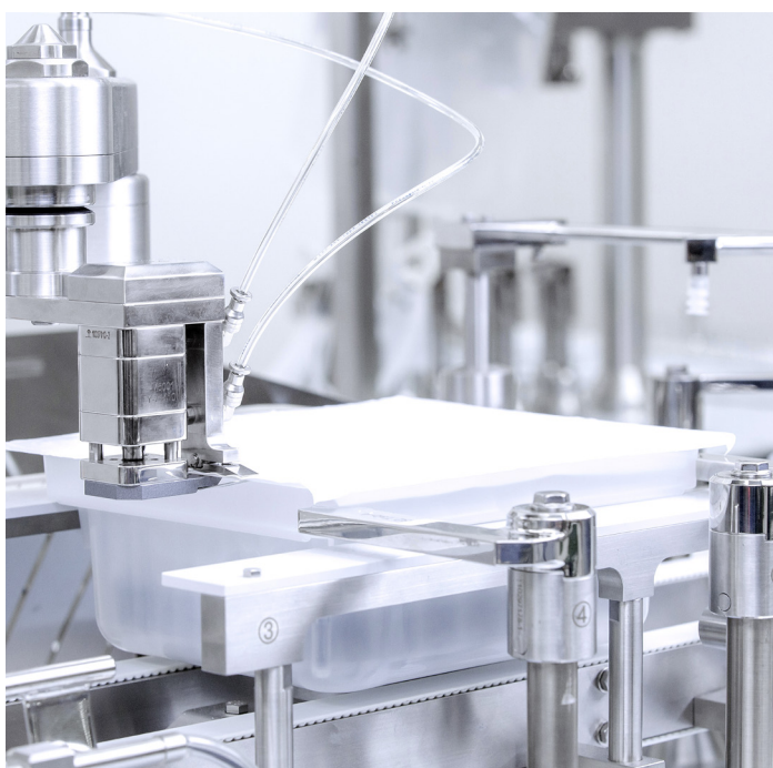
A tub of nested, sterile, ready-to-use containers, just prior to tub opening / lid removal. Image courtesy of Optima Packaging Group GmbH. Used with permission.
