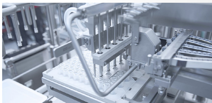
Filling and plunger placement of nested pre-fillable syringes as they reside in their nest. Image courtesy of Bausch+Ströbel. Used with permission.
