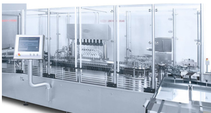
Vial filling and stoppering machine within a RABS enclosure. Note the opening above the RABS enclosure. The RABS enclosure is placed underneath filtered unidirectional air flow which is commonly provided by a separate air-handling unit. In order to allow the air to flow out of the RABS enclosure, the doors of the RABS enclosure have openings at the bottom. In this image, these openings can be seen guarded by stainless steel bars. Although not shown on this image, RABS enclosures may be outfitted with glove ports to allow the operator to make manual interventions without opening the RABS doors. Image courtesy of Bausch+Ströbel. Used with permission.
