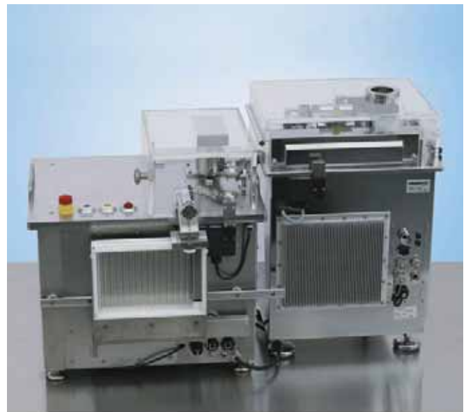
Figure 1: TANDEM is an on-line pharmaceutical tablet characterisation tool, which incorporates the Sotax 10X conventional tablet tester and Bruker's MATRIX FT-NIR spectrometer
