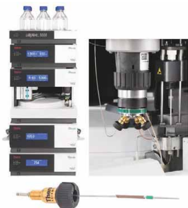
Figure 2: UltiMate 3000 BioRS system, detail of the autosampler inert injection valve, and the Viper connection.
