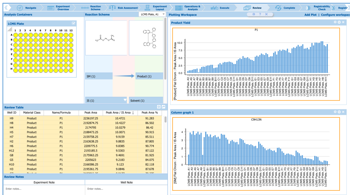
Figure 7: The plotting workspace further helps in the identification of the optimal reaction conditions suitable for scale-up. This plot shows product yield (top right) and residual starting material (bottom right) for the entire 96-well plate.
